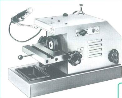
This machine is used to grind and lap carbide-tipped scraper blades, changing inserts, turning tools, reversible inserts, etc.
